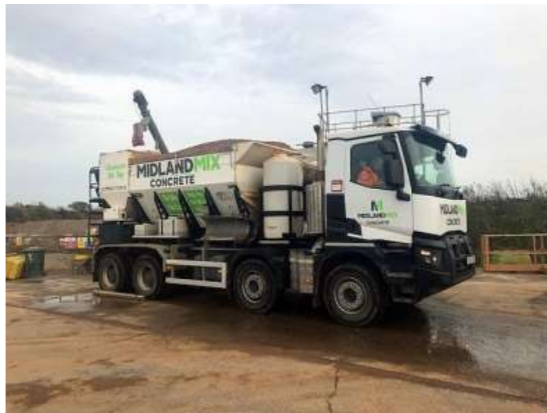
Figure 2 showing mixer lorry that are equipped to mix the concrete and keep it rotated and fresh until required – they will wait at the construction site throughout its nightly period of operation.
